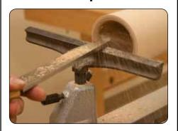
With a heavy scraper or hollowing tool, turn the remaining portion of the inside of the blank so it matches the taper of the beverage mug.
