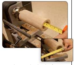
Make sure the depth of your hole is correct and mark a 2-15/16" diameter circle on the open end of the blank. This is your finished inside diameter of your wood sleeve.
