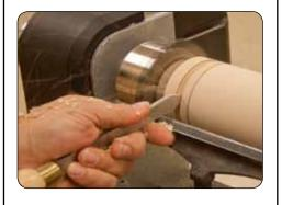
With the parting tool, start a parting cut on the left side of the mark to about 1/2" deep. This is your reference to the bottom of the mug. (see diagram on page 4)
