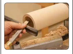
Working from the open end, turn the upper portion of the sleeve flat to the 2-15/16" diameter mark approximately 1-7/8" into the sleeve. (see diagram on page 4)
