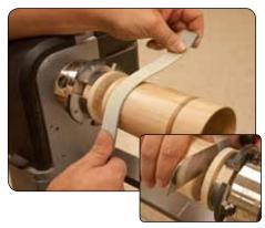
Sand the mug through 320 grit. Finish the parting cut at the base to about 1" in dia. The cut is typically made at a slight angle to give you a slightly undercut base. With the lathe turned off, remove the mug with a fret saw - sand off excess.
