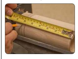
Measure the depth of your hole in the blank. Add a minimum of 3/8" to the depth and make a mark on the outside of the blank.
