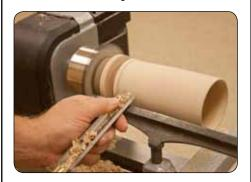
Turn your blank to shape. Make sure you leave a shoulder on the top side for the mug to register. This provides a nice, clean transition from the stainless steel to the wood.
