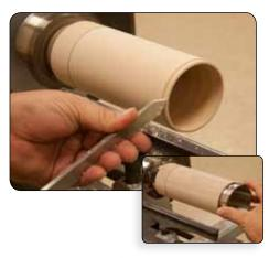
For the lip of the mug, turn a 1/4" rabbet on the top of the blank (with lathe power off). Check as often as possible to ensure a proper fit with the stainless steel insert.
